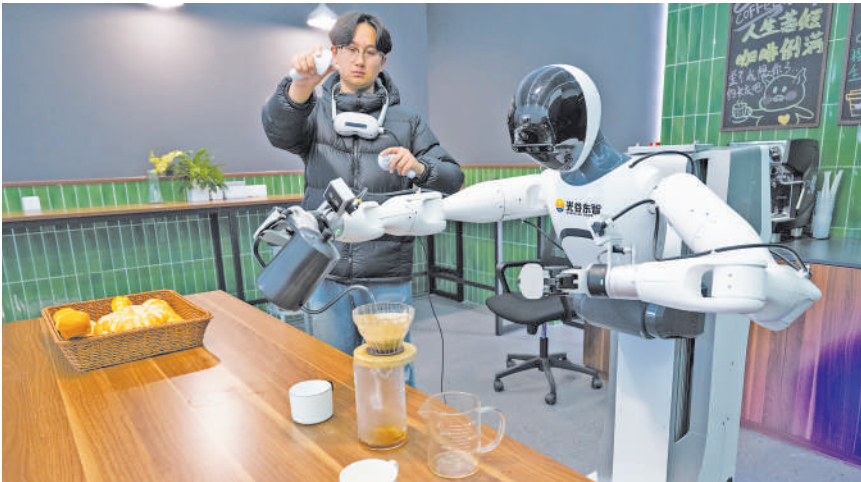
A staff member operates a robot to collect data in a coffee shop scenario at a humanoid robot innovation center in the Wuhan East Lake High-tech Development Zone in Wuhan, central China's Hubei province. (PHOTO: XINHUA)
