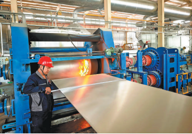
A worker at the aluminum sheet and strip production line in Minhe's industrial park, Qinghai province. (PHOTO: ZHANG Tianfu / Science and Technology Daily)
